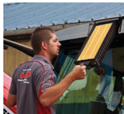
The cab air filter can be removed easily for cleaning
