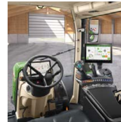
Profi Setting 2 - 3L joystick - 1 linear module (rocker pair) to control hydraulic valves - 12" terminal
