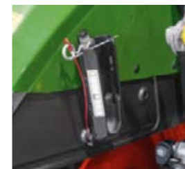
Safe storage location: the fully integrated ball holder on the inner mudguard.
