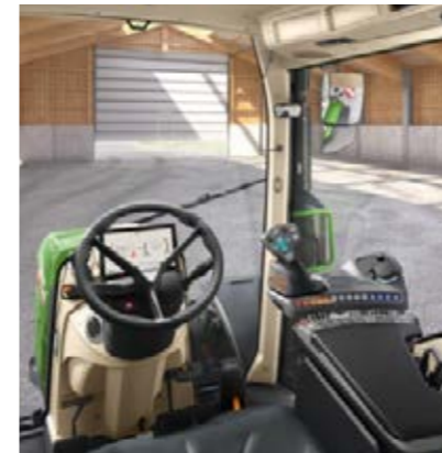
Power Setting 1 - No crossgate lever - 1 linear module (rocker pair) to control hydraulic valves
