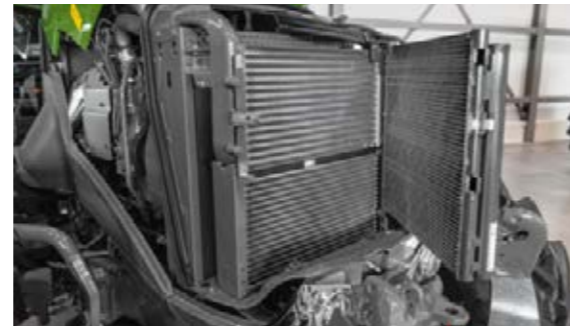
Less effort: The compact radiator package is very accessible and can be cleaned easily and quickly because of the generous clearance between the coolers and the flat radiator bottom.
