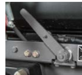
Prevents misuse and damage to attached implements: secure the lower link with the shut-off valve.
