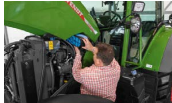
The high-performance air filter achieves optimum air intake and cleaning and is easy to replace.
