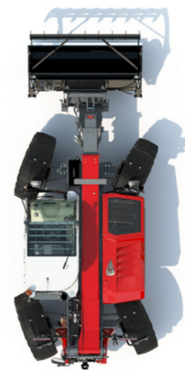
FOUR-WHEEL steering mode – for minimum turning circles.
