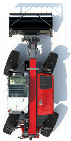
CRAB-STEER mode – for efficient filling and grading alongside walls in confined spaces.
